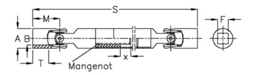
F = 25 Longitudinal ribs = 6x28x32M = 66MD max N m = 120
